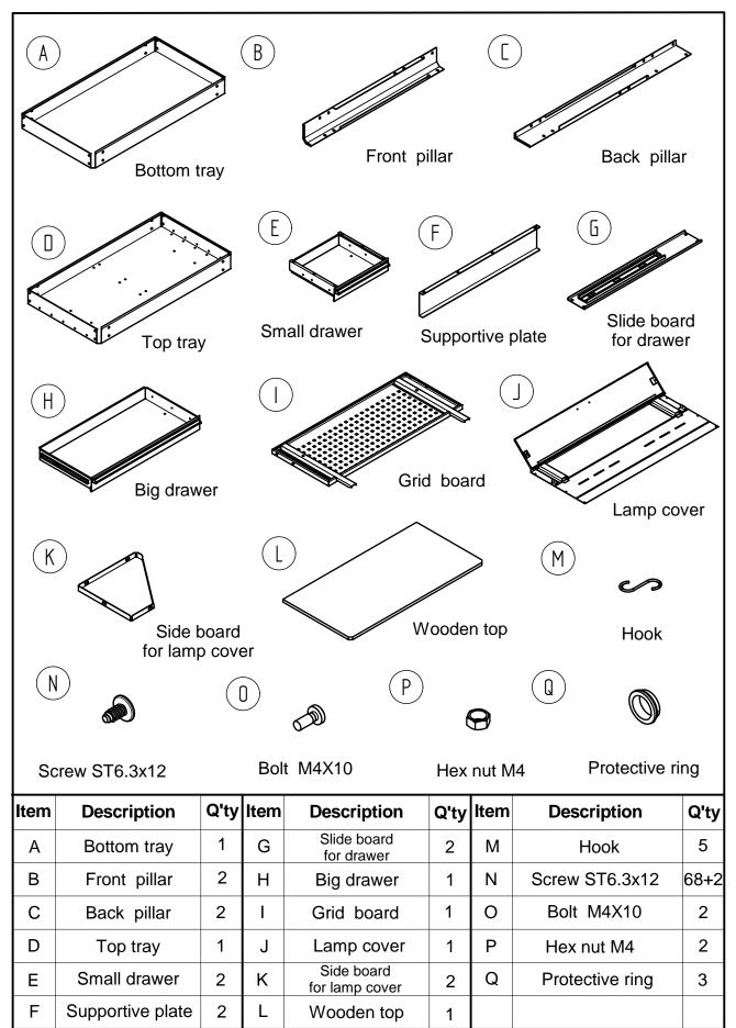
During assembly do not tighten bolts until all components are aligned properly, then tighten fully.
