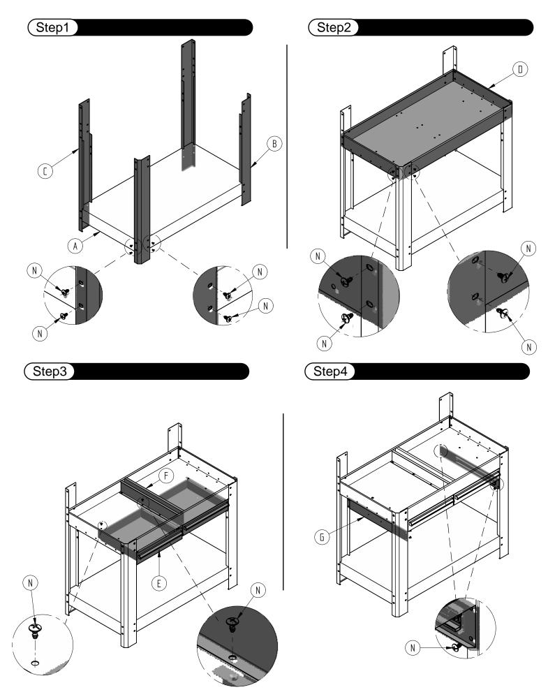
During assembly do not tighten bolts until all components are aligned properly, then tighten fully.
